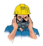
Gently place your palms over the cartridges/filters. Try not to press so hard that the fit of the facepiece changes on your face. If you can't completely cover the cartridges/filters with your palms, you can perform the test by covering the cartridge/filter with a thin nitrile or latex glove.
