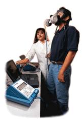
machine monitors the levels of harmless particles inside the facepiece of your respirator and compares them to the levels of harmless particles in ambient air around you - the lower the levels of particles inside your mask, the better the fit. During your fit test, you will be asked to perform some activities while wearing your respirator (e.g., breathing normally, breathing deeply, talking, bending at the waist).
